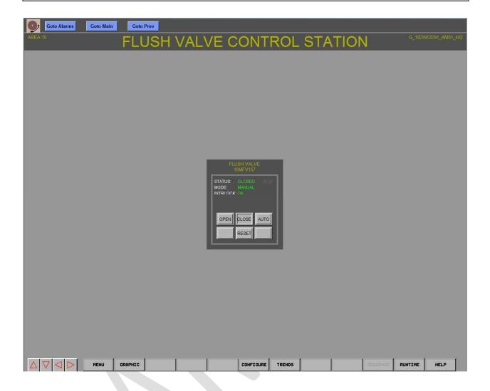
This screen shows OPEN/CLOSE/AUTO control of the flush water solenoid valves The operations of these components are described in the component subsections of this memo.
