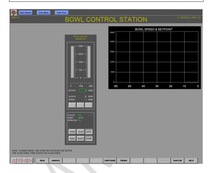
This screen shows START/STOP/AUTO control of the bowl motor. The operations of these components are described in the component subsections of this memo.
