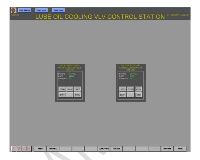
This screen displays the control stations for the liquid side and solid side pumps associated with the centrifuge lube system. The operations of these components are described in the component subsections of this memo.
