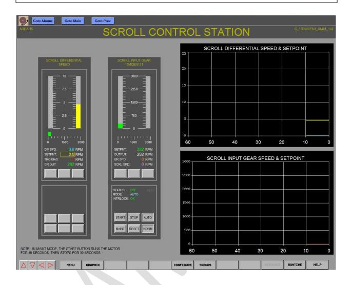
This screen shows START/STOP/AUTO control of the scroll motor. The operations of these components are described in the component subsections of this memo.
