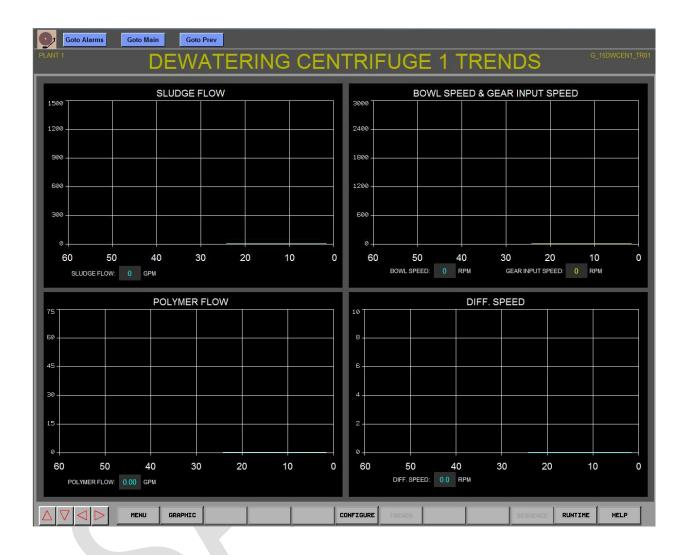
This screen displays the trends centrifuge sludge flow, polymer flow, bowl speed and gear speed, and differential speed.
