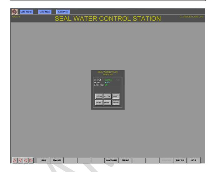
This screen shows OPEN/CLOSE/AUTO control of the seal water solenoid valve. The operations of these components are described in the component subsections of this memo.
