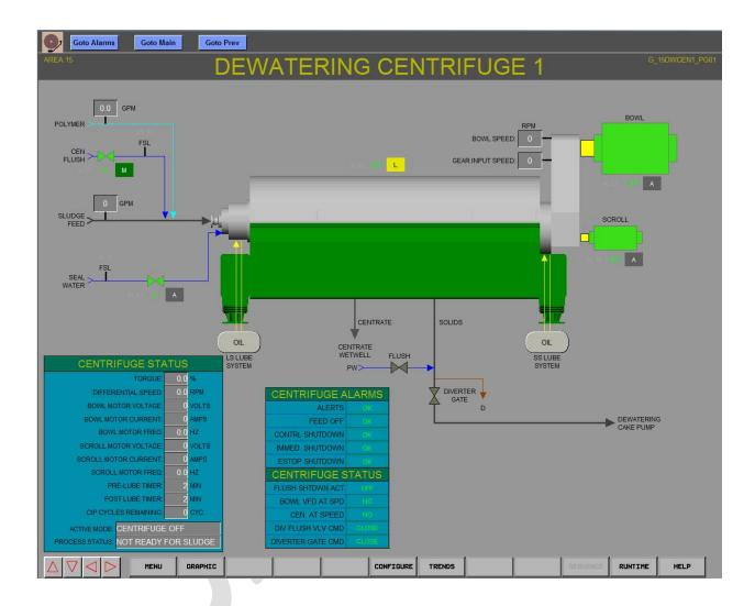
This example screen shows several conditions which could exist for the centrifuge, but would not necessarily exist simultaneously.
