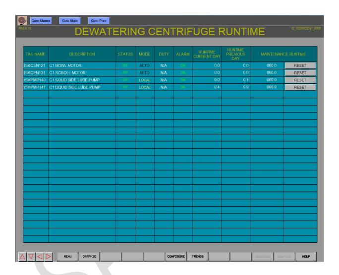
This screen displays the runtimes of the equipment along with status, mode, and alarm condition. For this system Duty (Lead/Lag conditions are not applicable).
