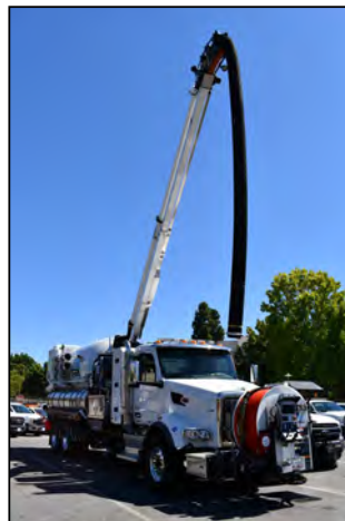
View of Vactor Truck with Extended Hose
