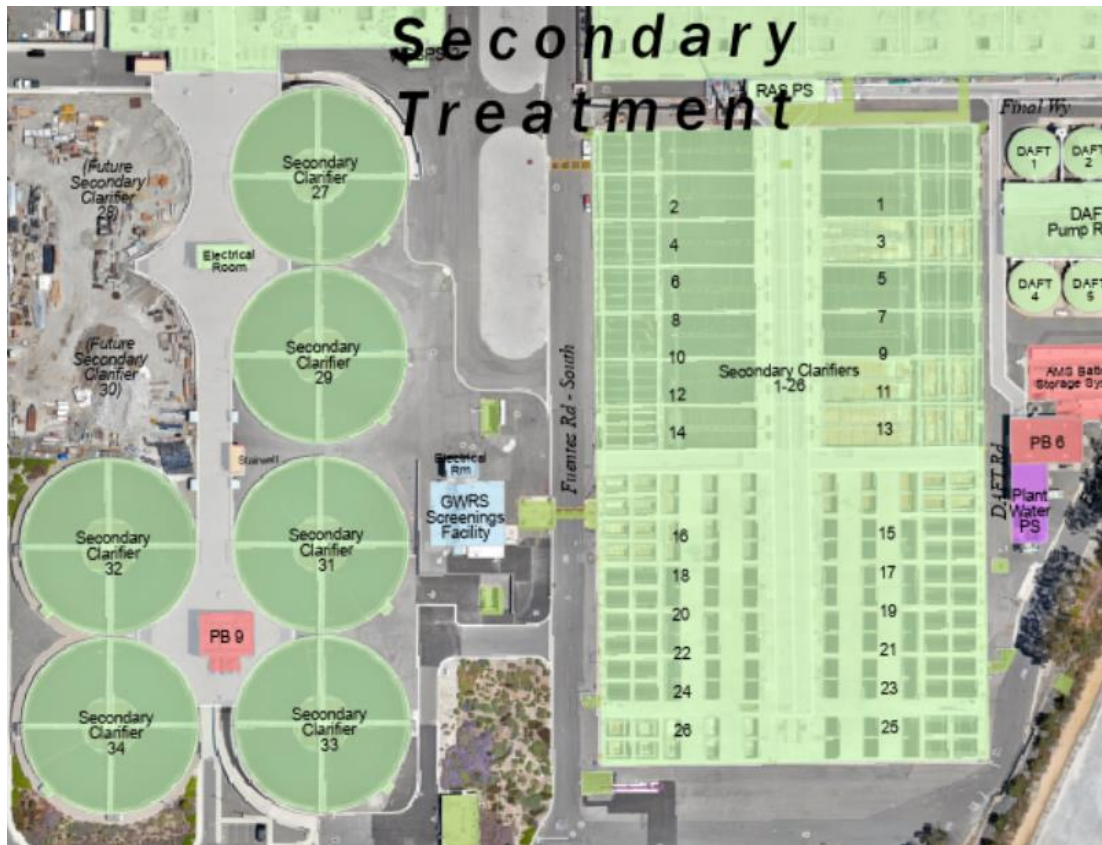
Figure 10 - Secondary Clarifiers Nos. 1-26 (odd) currently feed into the PWPS.
