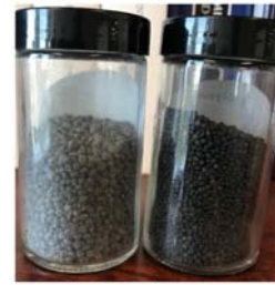
Biosolids Pellets from dryer
