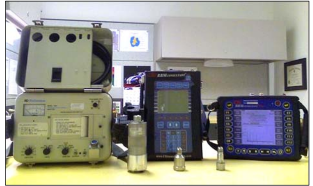
Figure 4-6. Vibration Analysis Equipment
