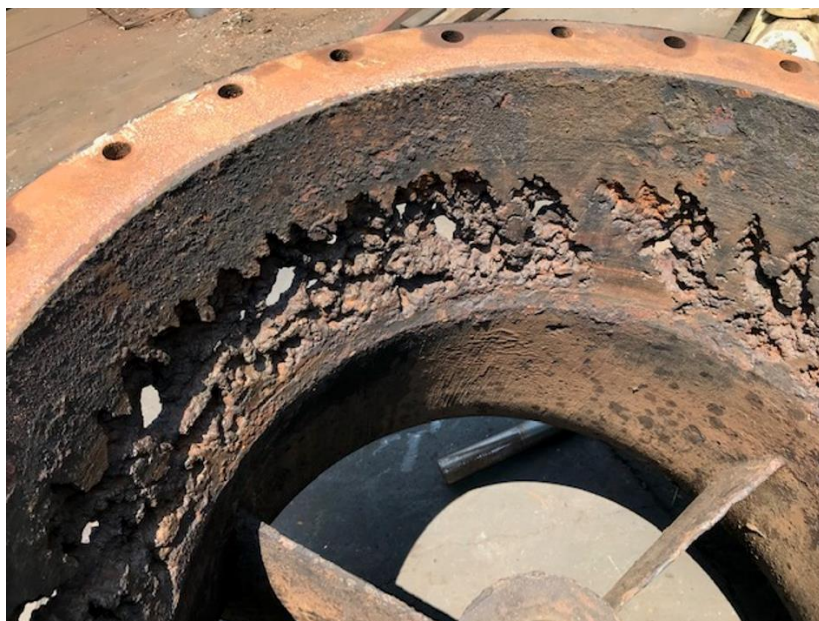
Figure 2: PEPS Pump No. 4 Impeller showing signs of heavy corrosion and in need of replacement.
