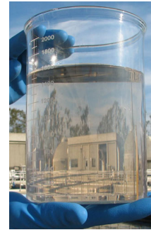
Secondary Treated Effluent
