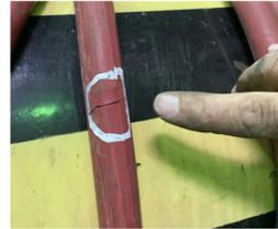
Cracked generator cable leads
