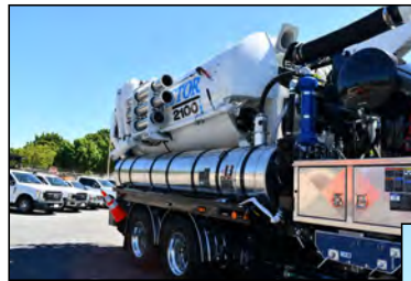
View of Debris and Water Tanks
