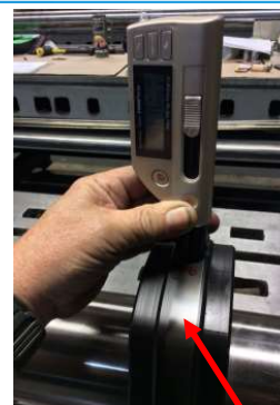
Camshafts worn; new camshaft lobes required
