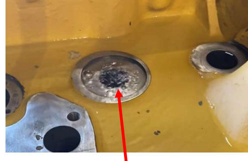
Failed hydro testing; bubbles should not be present
