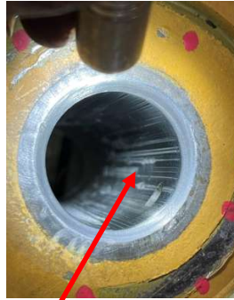
Damaged valve guides
