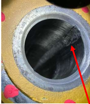
Damaged valve guides
