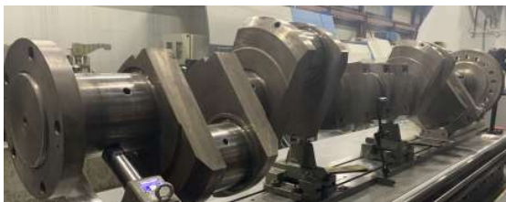
Crankshafts require straightening
