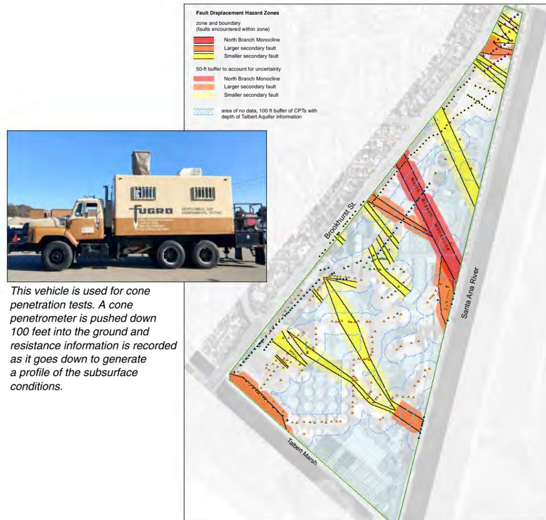
This vehicle is used for cone penetration tests. A cone penetrometer is pushed down 100 feet into the ground and resistance information is recorded as it goes down to generate a profile of the subsurface conditions.
