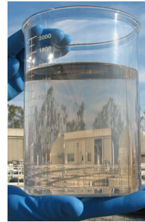
Secondary Treated Effluent
