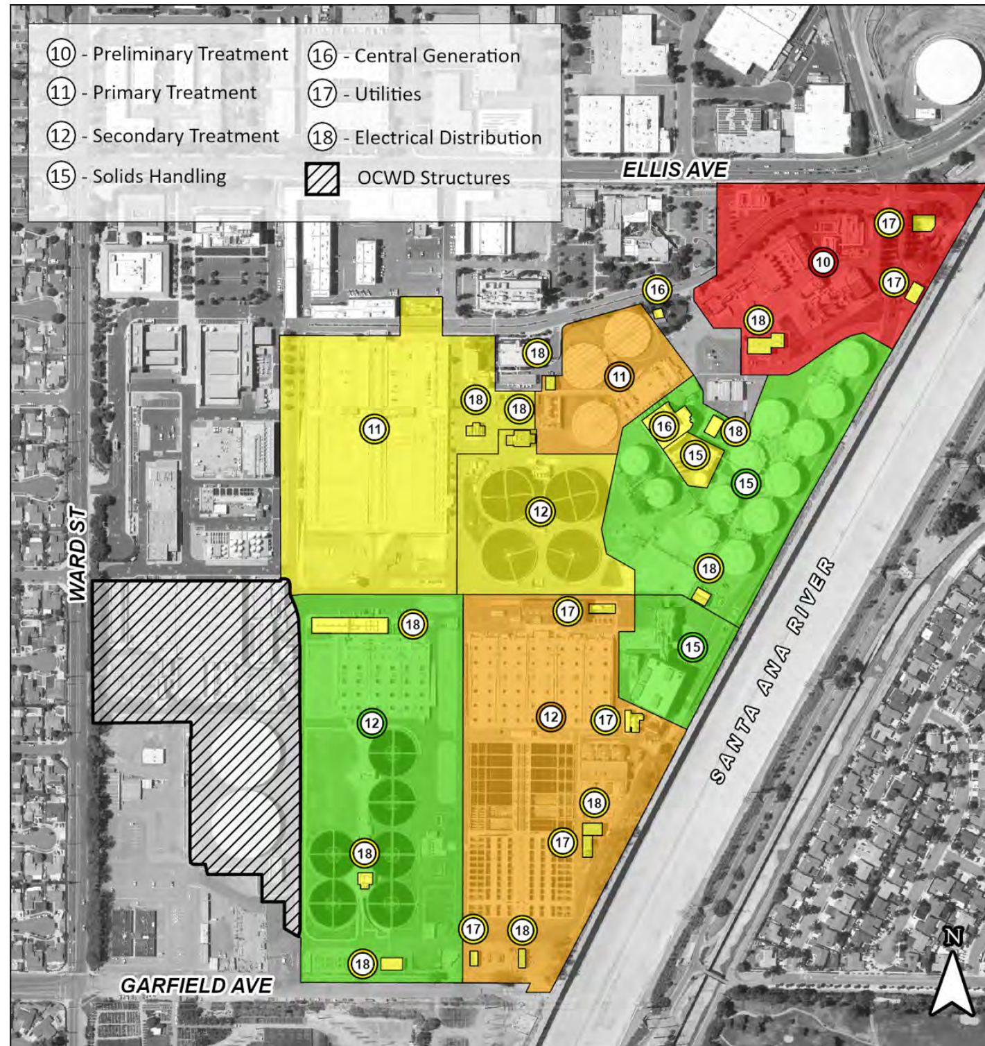
Figure ES-1-3. Plant No. 1 Process Area – Remaining Useful Life Score Map
