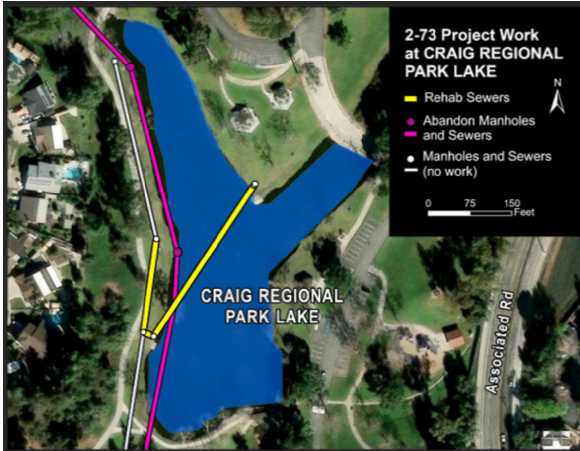
Figure 5 – In-Service Sewers and Manholes Rehabilitation within Craig Regional Park
