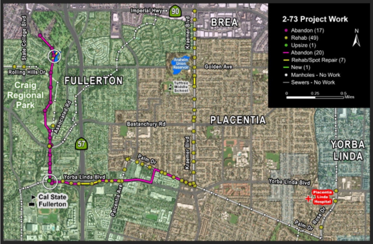
Figure 4 – In-Service Sewers and Manholes Rehabilitation Map
