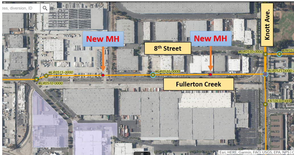
Figure 2. New Manhole Locations
