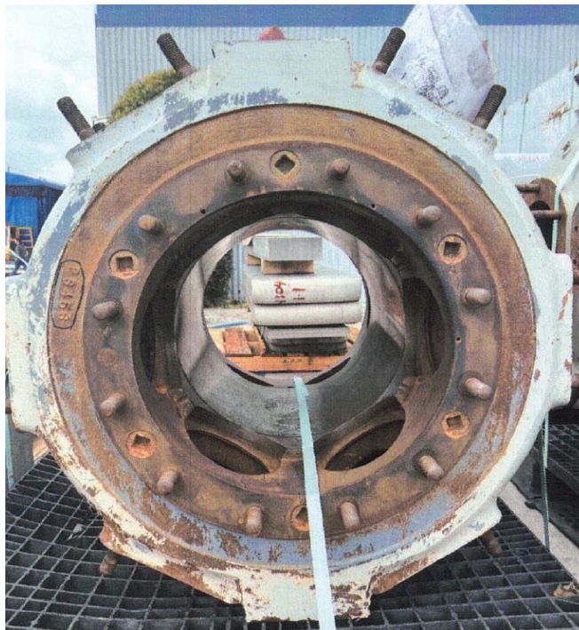
Figure 2: A Gas Compressor Cylinder showing signs of byproducts of corrosion and in need of replacement from a recent overhaul.
