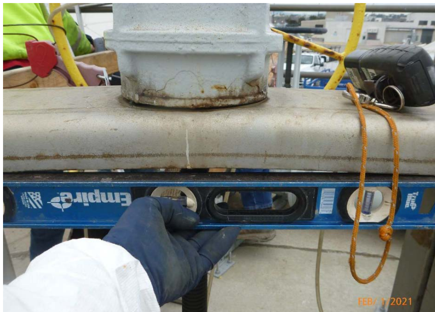
Picture 5: Bent gate top frame
