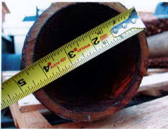
Corrosion is evident in this wastewater pipe from Los Angeles County. (Image: Los Angeles County Public Works Department)
