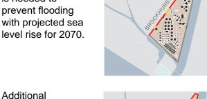
floodwalls along the Talbert Channel and Santa Ana River will protect Plant No. 2 from flooding due to maximum tsunami risk for the region.
