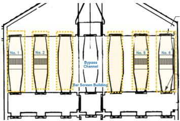
5/8" Spacing 1" Spacing Refurbish 4 existing bar screens
